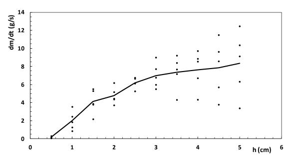
Figure 3. Mass of embers that transposed the gap as function of gap height h (cm). The continuous line is the average of five tests.
