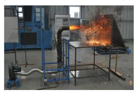
Figure 1. Firebrand Generator Device
