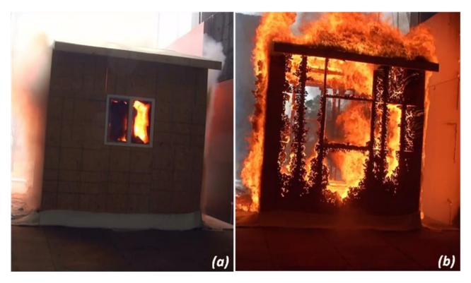
Figure 6. An example of real structures tested used in similar studies (a) after 4 minutes (b) the same structure after 10 minutes (source NIST, 2013)
