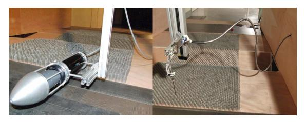
Figure 4. LDV on the left and FID on the right above the V-shaped forest model
