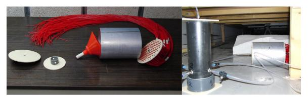
Figure 3. The two photographs depict the distribution device of ethane placed under the model
