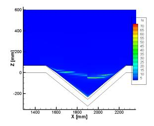
Figure 7. Turbulence intensity on U for  $\alpha = 50^{\circ}$
