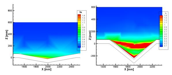
Figure 6. Turbulence intensity on U for  $\alpha = 80^{\circ}$  on the left and  $\alpha = 50^{\circ}$  on the right
