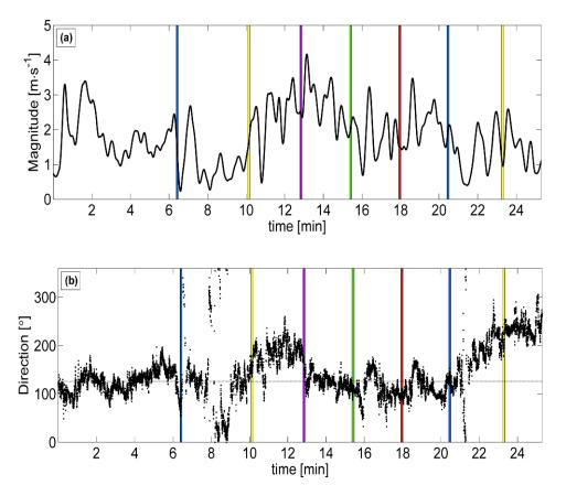
Figure 4. (a) Magnitude and (b) direction of horizontal winds at the sonic anemometer on the Overstory Control tower. Colored lines correspond to the time of fire contours P2-P8 (refer to Figure 2). Time is given in minutes from the start of ignition. Direction is given in compass degrees (clockwise from north). The horizontal line in figure (b) represents the general direction of fire spread.
